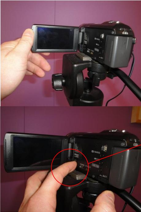
Insert the plug into the socket.
