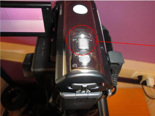
Use the W – T switch on top of the camera to respectively turn the volume down or up.
