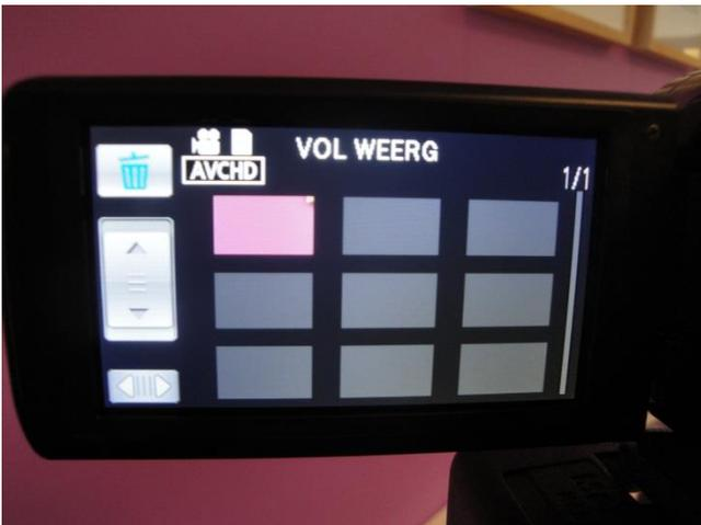
To remove clips, make sure the camera is not connected to laptop or PC. Switch the mode switch to the
