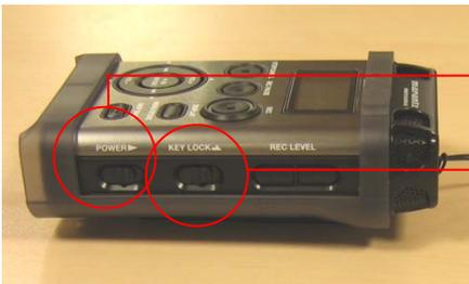
Move the POWER button to the side, hold for a moment, then release to turn the device on. The same procedure goes for turning the device off.
