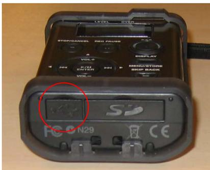
Open the hatch marked with the USB icon (🔌) on the bottom of the device. Insert the USB cable into the USB socket of the voice recorder. Insert the other end into one of your PC's/laptop's USB ports. Make sure the voice recorder is on.
