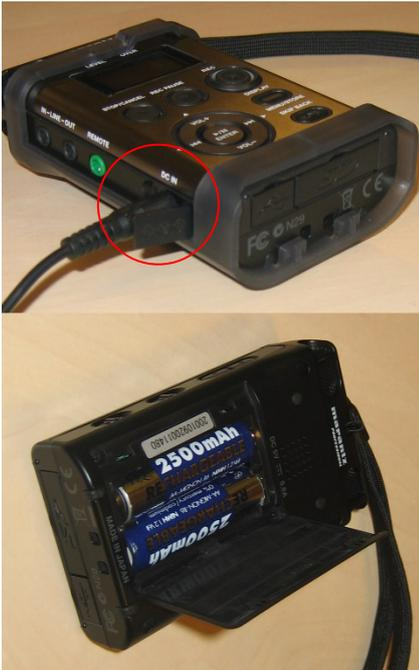
Plug the power connector into the DC IN input of the device. Plug the other end into a power socket.
