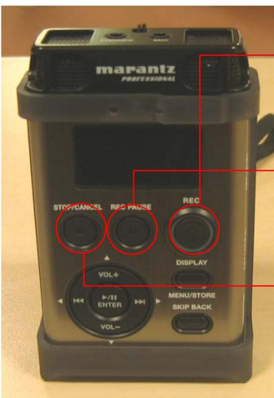
Press the REC button to start recording. The timer on the display will start running.
