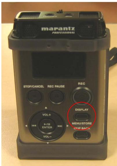
Make sure all files are deleted from the voice recorder before returning. To delete all files, turn the device on and go to the menu by holding the DISPLAY-button. By using the VOL+ and VOL- buttons, scroll through the menu to option 5: Utility.
