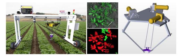
We would like to develop a delta manipulator that is suitable for the heavy agricultural environment. This includes the wet, sandy environment where crops are grown. The manipulator will be part of a total system as shown in the first figure above. You will start by drawing up the requirements, defining functionalities, coming up with solutions, after which a concept will be developed into a prototype.
